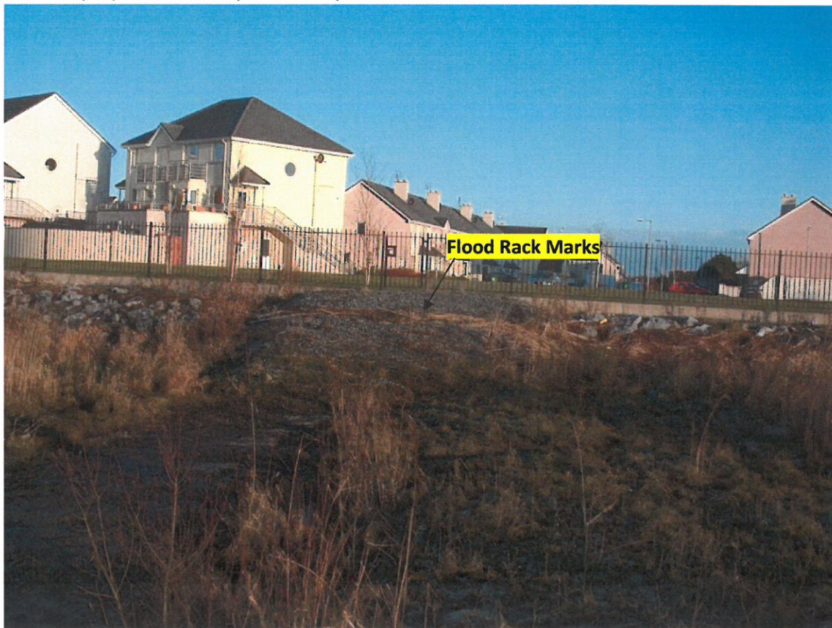
Plate 8 November 2009 flood event Rack Marks from River Fergus Surveyed by Hydro Environmental Ltd at 5.95mOD located upstream of Gort Road Industrial Estate and adjacent to Ard Caoin Housing Estate.
